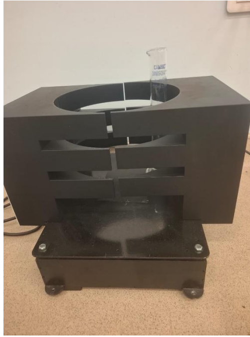
Figure 17. Compressing the powders in a vibrating machine.
