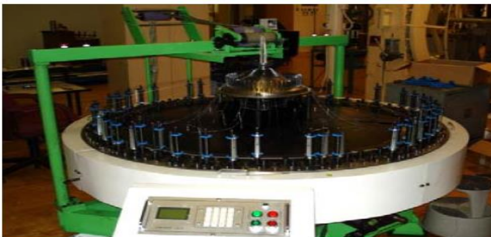
Figure 5. Lace braiding machine [2]
