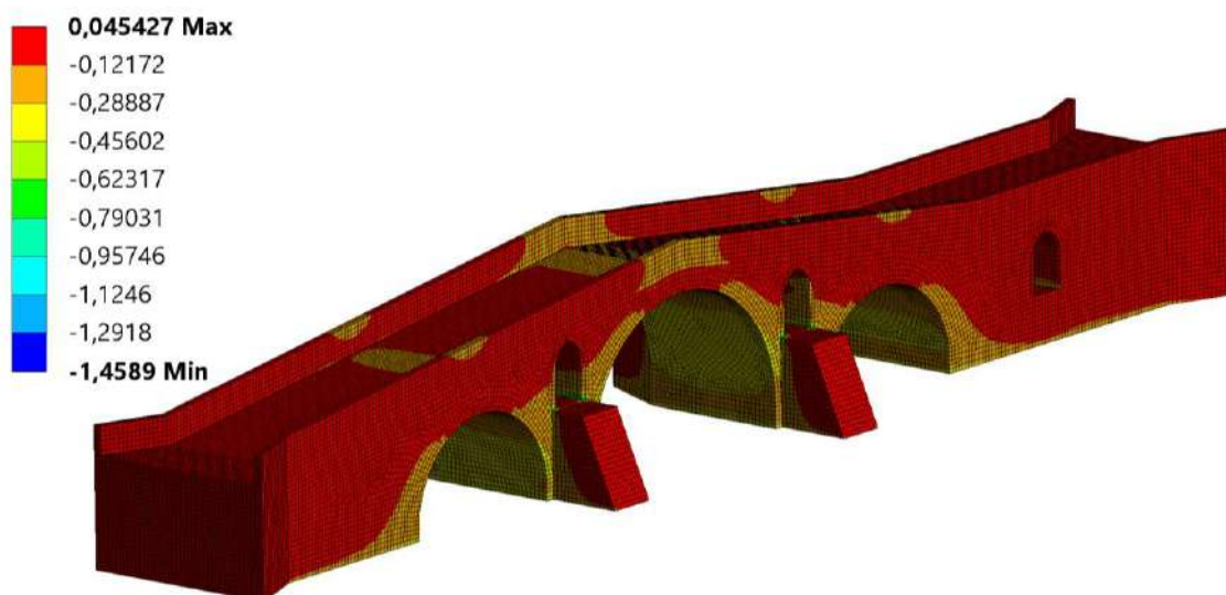
Fig. 6. Minimum principal stress obtained from the static analysis
