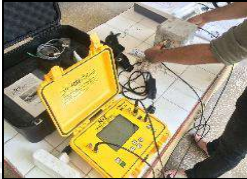
Figure 2. Ultrasonic Pulse Velocity test device
