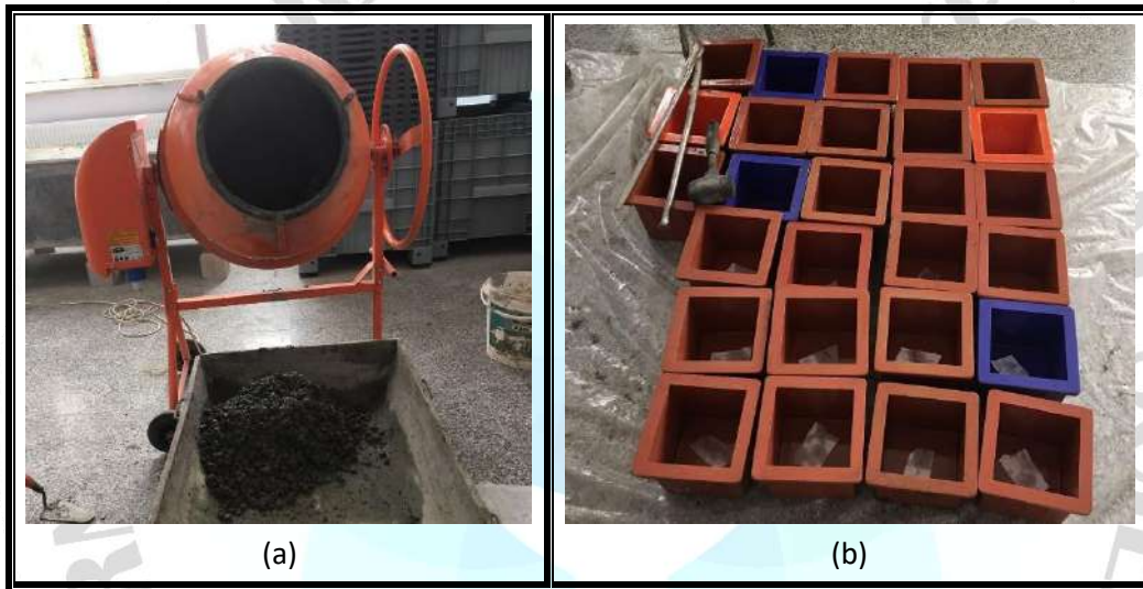
Figure 1. a) Laboratory type mixer b) The molds filled with fresh concrete
