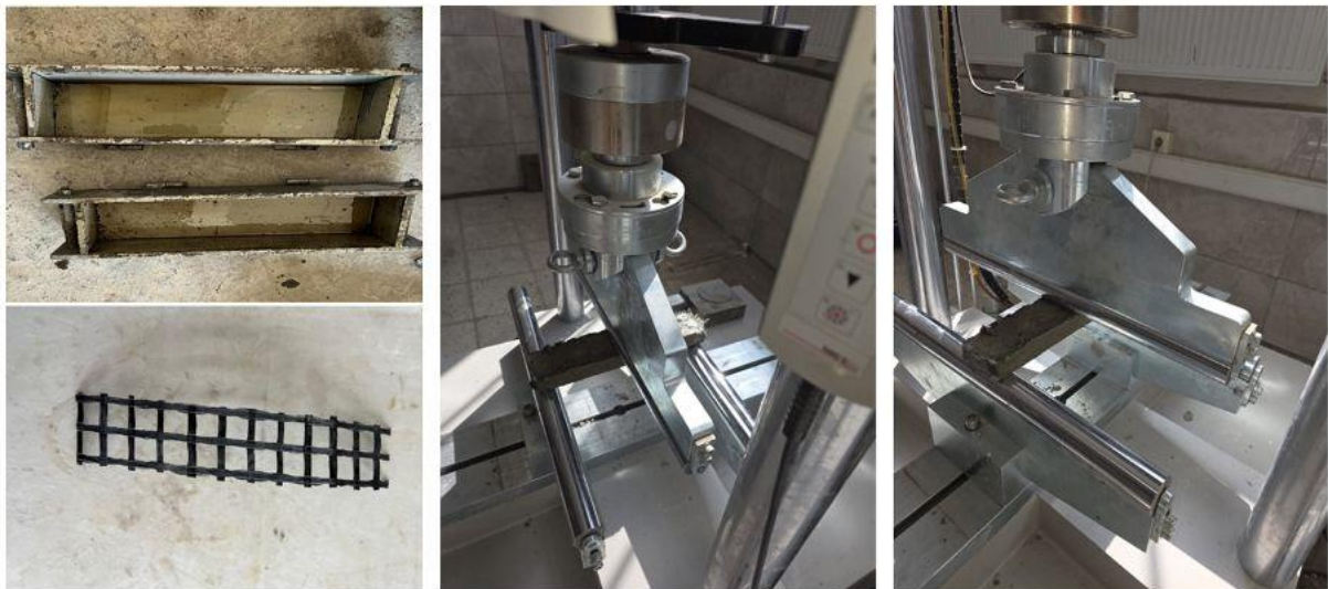
Figure 5. (a) Beam specimen molds and carbon mesh, (b) and (c) experimental setups.
